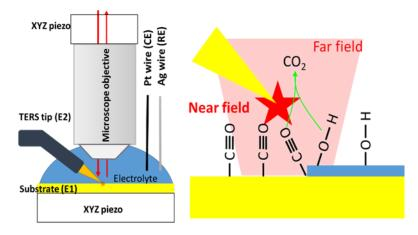
Principle of electrochemical TERS and schematic of measurements that will be performed.
