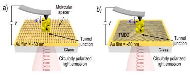
a) A chiral plasmonic nanocavity is formed between a chiral gold nanoparticle and a thin gold film. When a voltage difference is applied between the particle and film via the tip of an atomic force microscope, the resulting inelastic tunneling electrons excite the existing plasmonic modes of the system (which subsequently decay as circularly
