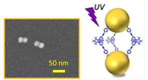
Assembly of gold nanoparticle dimers, connected with switching molecules (Electronic Microscope images and scheme). Switching from conductive to insulating states of the molecules is triggered by light and will be measured with a conductive AFM.
